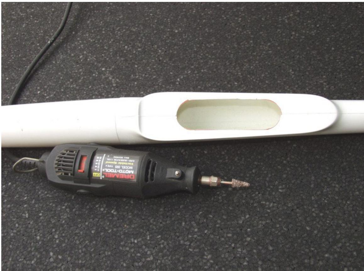
*Dremel fitted with Permagrit cone, makes light work of this chore*
