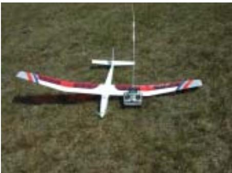
Using the included propeller setup, the model climbs out quite well at an angle of around 30 degrees and motor run times are around 10 to 14 minutes. This time can be extended when a thermal is encountered, and the glider climbs strongly. Switch the motor off and enjoy the experience.
