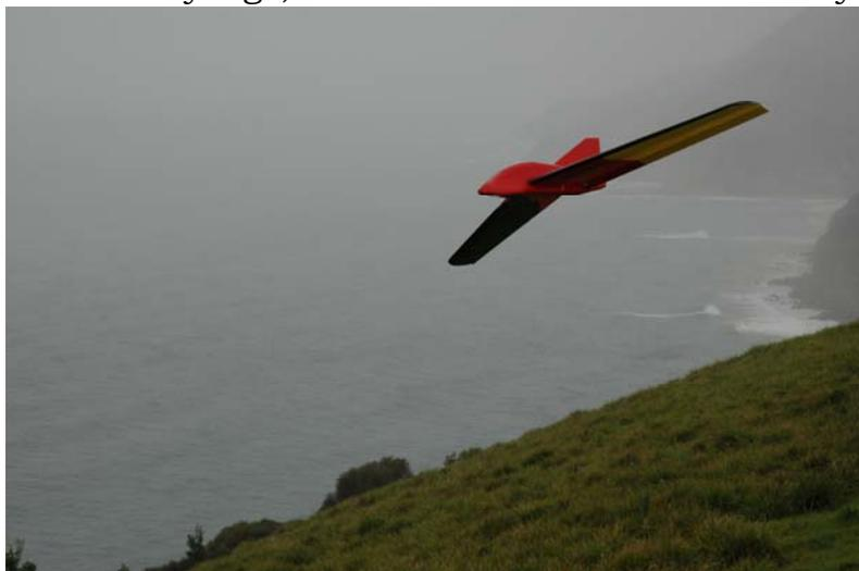
A reasonable day finally came, and the Arrow was tossed off a slope which is only around 12m high, and where the ocean is only around 30m away. A firm toss and it ballooned up, almost into a stall. A bit of down stick and it sailed out straight and level. It needed only 3 clicks of down trim to see it right. The Arrow was quite
